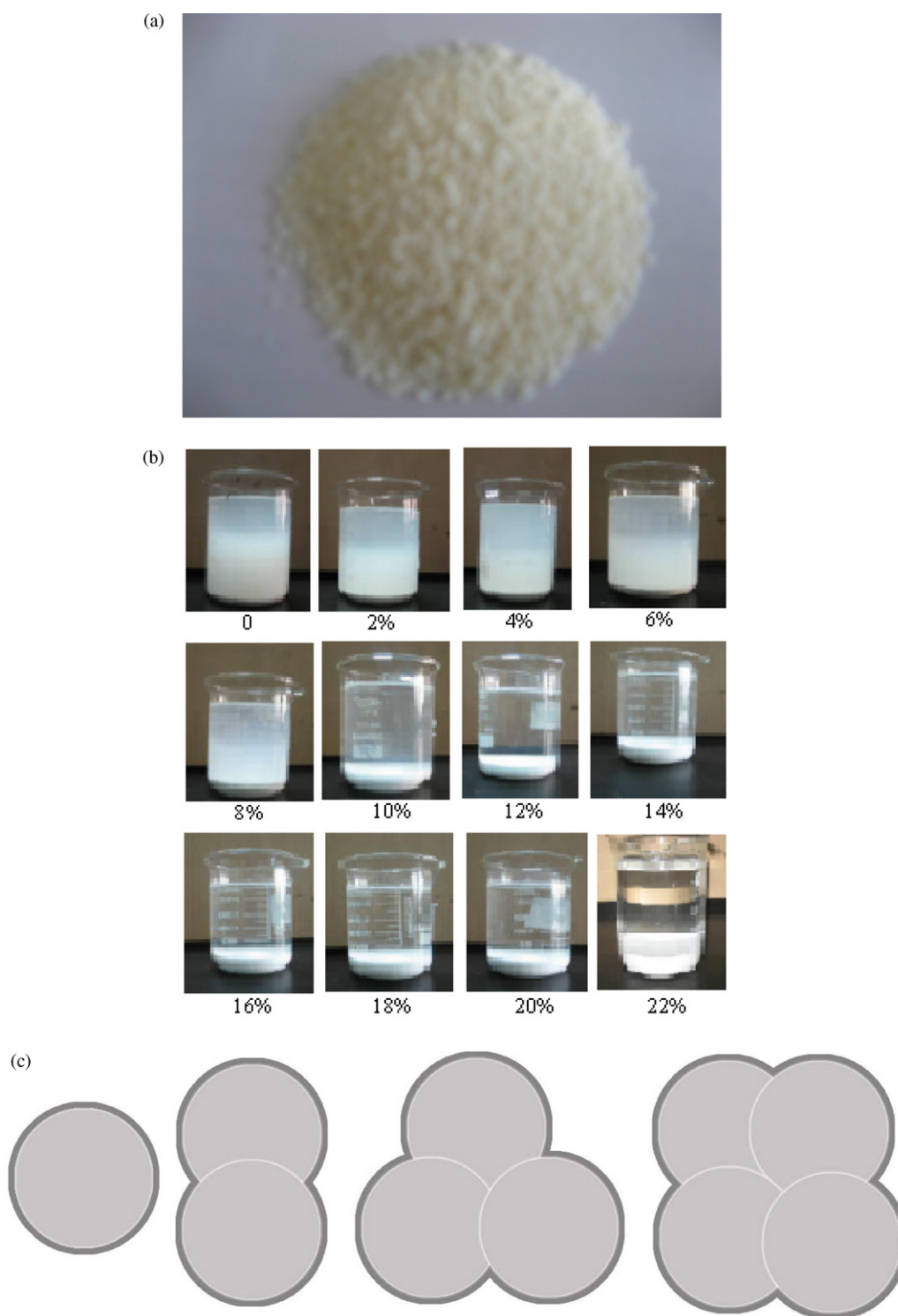
Fig. 1. Macroscopic optical photographs of (a) carboxymethyl cellulose and (b) modified filler slurries (at different alum dosages) taken with a digital camera (Canon), and presumed illustrative structures of the modified filler particles at high alum dosages of above 10% (c).
